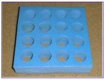
Similar results <u>might</u> be obtained with a hole saw (*without* the center drill bit) running at very high speed. I did not try that method. *Do not attempt drilling foam with a twist or spade drill.* It will just wrap the foam onto the drill bit and could cause injury if your are holding the work by hand.
