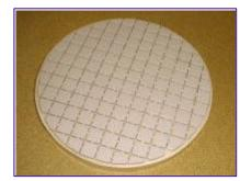
After the wax has cooled to room temperature, you may remove the tool from the mirror by gently sliding the aluminum foil off. Once off the mirror, carefully strip the foil off the tiles. It should come off without much trouble since little wax generally seeps under the tiles. Check to be sure that the wax created good adhesion between the window screen and the plaster base. Check also for voids around the edges of the tiles where the tool might not have been pushed into the wax far enough.
