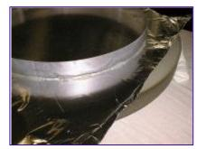
If you choose do not use hot melt glue, you may also use modelling clay or just place small pieces of tape at 0.5" intervals all around the dam to make sure it doesn't lift when pouring the plaster. (I am quite a fan of hot melt glue. I have found a multitude of ATM uses for it over the years. The "hot glue guns" are quite inexpensive and the glue is also very cheap. If you have never tried using it, you should.)
